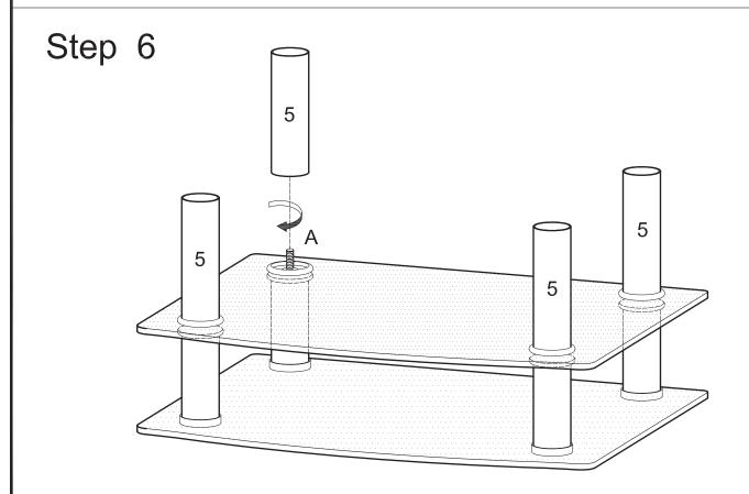
Screw cylinders (5) onto long rods (A). Note that cylinders (5) will fit snuggly inside the decorative rings placed in the previous step.
